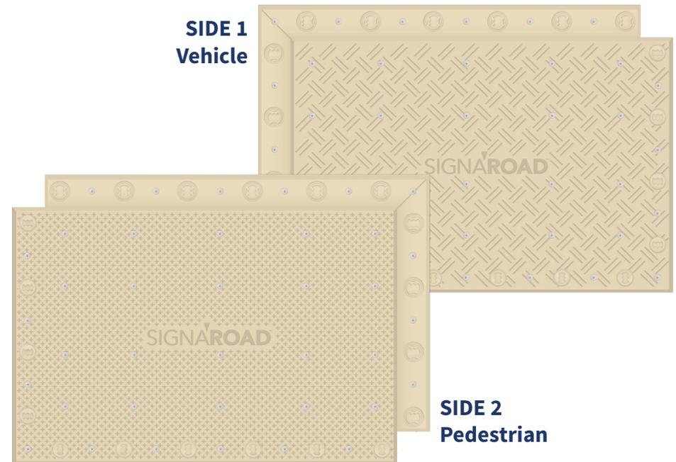
SignaRoad mats incorporate overlapping flanges on both sides that allow mats to connect to adjacent panels. Flanges are solid HDPE for added durability. Each flange incorporates a heavy radius design, providing additional strength and shear resistance. Once nested into adjacent panels, the solid HDPE flange system provides rigidity and strength.
